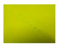
**PVC** was put under the same test as **micrAgard**. The surface of the material was scraped off and it lost all of it's properties as the surface had been tampered with. Once the surface is damaged bacteria can infest the material and remain there for it's life-time.
