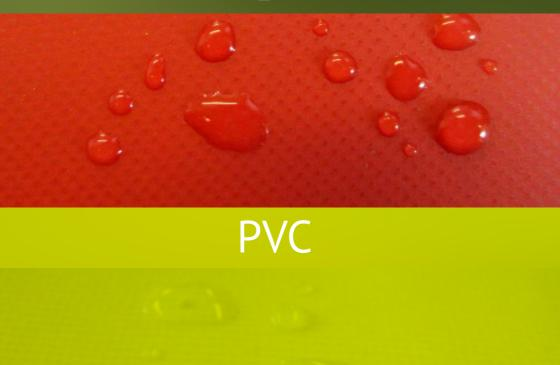
The same test was also done on the material swatches which had been put through the abrasion test; all the moisture soaked into the PVC fabric whereas the micrAgard left the water on the surface.
